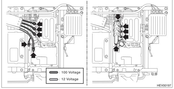
(3) Remove the bus bar from the drive motor inverter amperage sensor.
